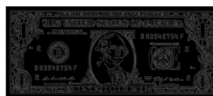
Figure 9: Canny Filter darkened the image, making the edges white thus greatly contrasting the two
