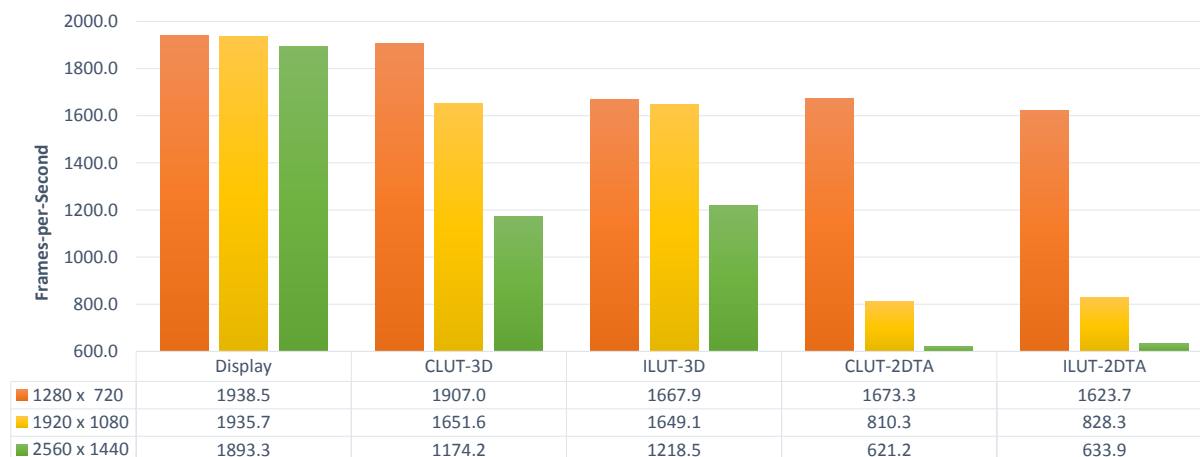
Figure 8: Performance of GPU-based LUT mapping performance in FPS for different LUT representations compared to a pass-through display pass.
