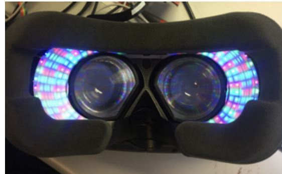
Figure 3: HTC Vive with a Sparse Peripheral Display extending the FOV to 180°.
