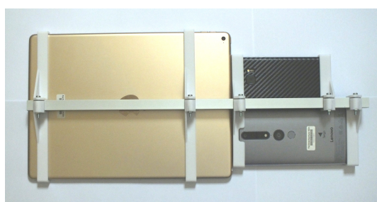
Figure 5: Test setup for fixing the devices. For testing purposes we added a Google Tango device, a now abandoned AR-project by Google that uses specialized hardware for tracking movement and the environment.
