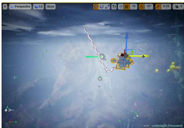
Figure 7: Experimental verification of motion of an extensible cable. We colored the cable in a checkers like pattern to enable the extension of the cable to be observable.
