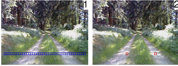
Figure 20: Find Tracks: Horizontal Scanline (1), Detected Tracks (2).
