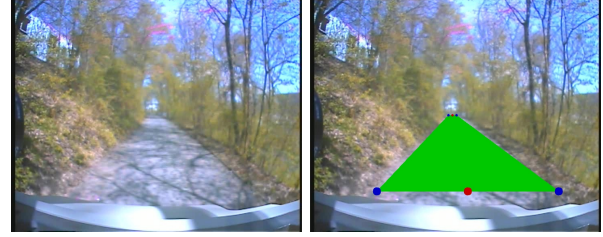
Figure 12: Polygon Fitting: Input(left), Resulting Polygon with auxiliary points(right).
