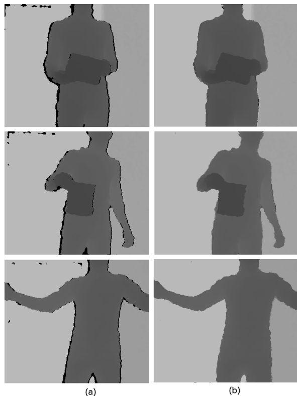
Figure 3: Results for our own datasets. (a) original raw depth images. (b) depth images enhanced by our approach.
