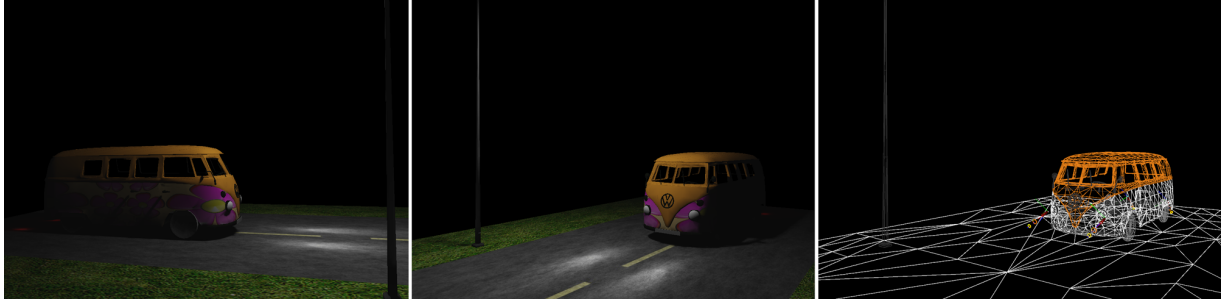
Figure 8: The scene consists of 9012 triangles which are divided into 4259072 elements. The street lamp is simulated with a standard Lambertian light, the head and taillights are simulated with four spotlights. Each triangle was assigned a 32 \times 32 radiosity texture and shooting was done from the third mipmap level.
