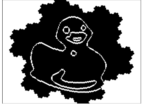
Figure 11: Edge map by thresholding the Gaussian blurred image at level 32.
