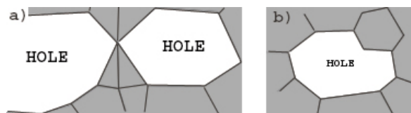
Fig.2 Two cases of holes. a) shows two connected holes and b) shows a single polygonal hole.
