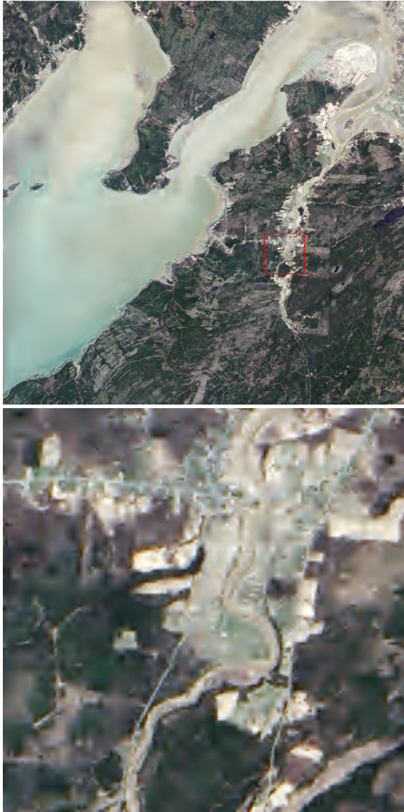
Figure 8: Drastic compression (34:1) of a 3000 \times 3000 pixel aerial image. The marked area is magnified below the full image.
