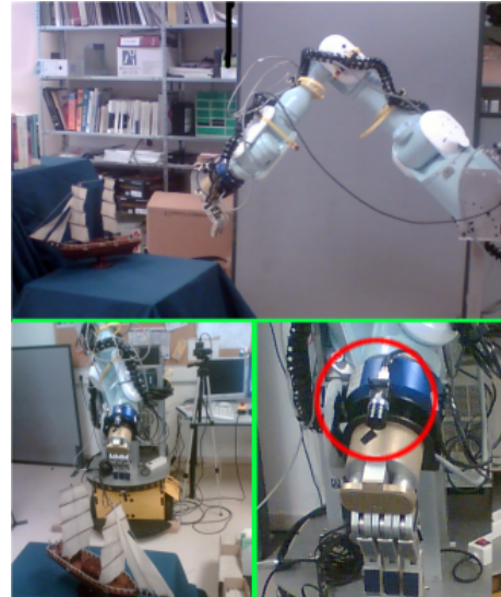
Figure 2: The robot arm is controlled by a PC. The arm is moved to different locations and takes snapshots of the object to capture.
