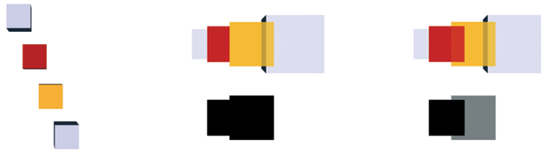
Figure 2: The figure shows a small setup of four boxes, whereby the light blue are unimportant objects and the orange / red boxes are objects of interest (left, shown from top). In the center, the conflict between the objects of interest is solved using standard depth sorting. At the right, gradual differences between the objects of interest ensure the visibility of the red box (importance maps are shown below).
