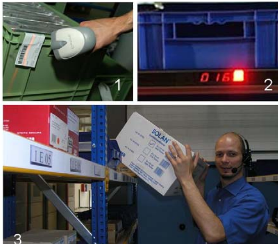
Figure 1: Order picking technologies: scanner (1), Pick-by-Light (2) and Pick-by-Voice (3)
