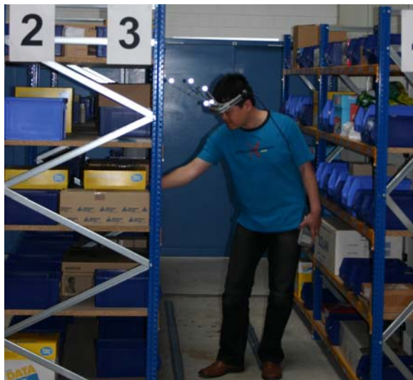
Figure 7: Pick-by-Vision including an infrared tracking system with targets fixed on the HMD
