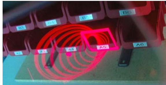
Figure 8: Frame and tunnel becoming transparent if the right storage compartment
