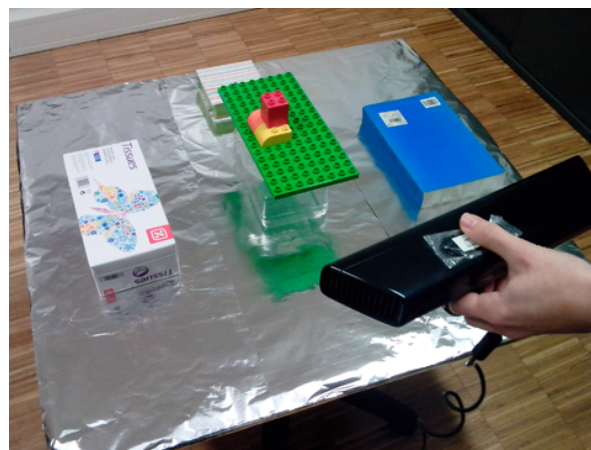
Figure 3: System setup. The object is created and subsequently positioned at the center of the table. Afterwards, it is acquired using one Microsoft Kinect ® and able to be processed.
