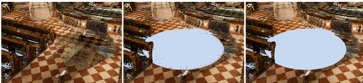
Figure 3: From the original point cloud (left image) a spherical volume is deleted. The center image shows the artifacts that remain when the interior nodes are not updated after deleting points. In the right image the points in the interior nodes have been updated according to the deleted volume.
