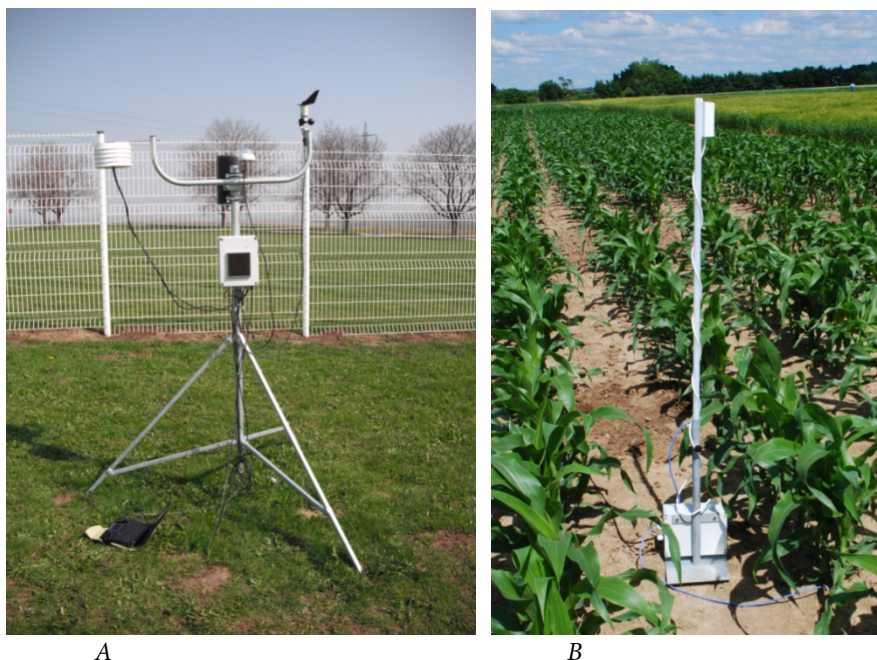
Figure 3. Meteorological station installed at the farm near to “Haj” experimental field (a) and sensor node installed in maize small-plot field at Field Experiment Station of Mendel University in Brno (b).
