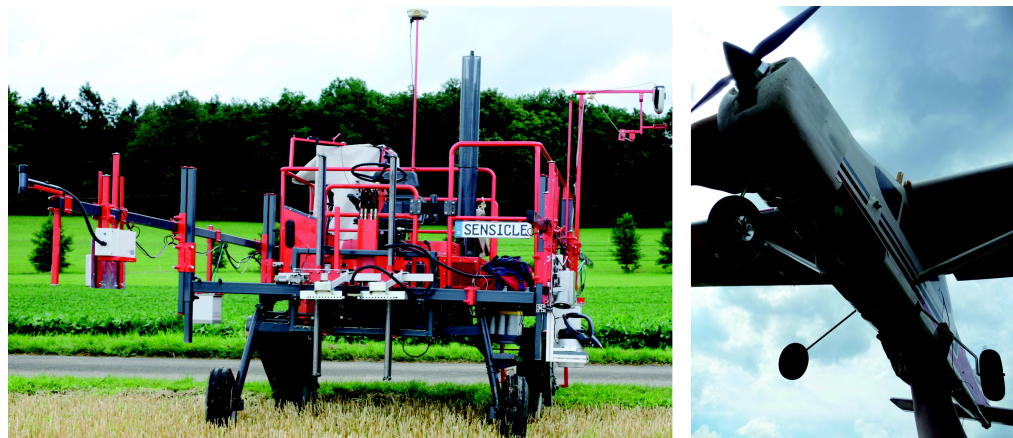
Figure 1. left: Sensor platform “Sensicle” for simultaneous field measurements with different sensors. The sensors are mounted at the left and/or right of the vehicle to be able to measure the same locations along the track; right: UAV with spectral sensor.
