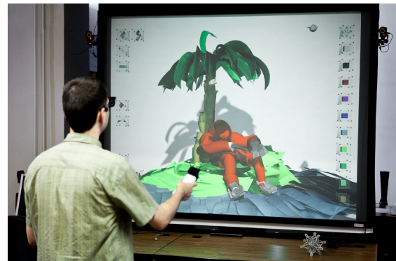
Figure 1: 3D painting in a virtual environment controlled with Wiimotes™, with position of user's hands being tracked by the OptiTrack™ system. The application was developed using the VRECKO system.
