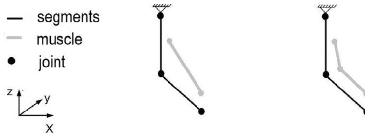
Fig. 3. Prescribing of the muscle course around the joint; muscle without prescribed course (left), muscle with prescribed course (right)
