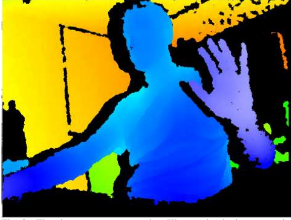
Fig. 3: The image represents the Kinect depth image, color represents the distance between camera center and distance plane. The black pixels have unknown depth value, mostly because of range constraint, occlusion or reflective surface material.
