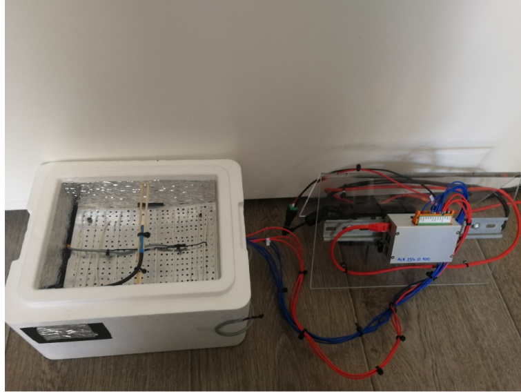
Figure 58: Open incubator with the Monarco HAT and Raspberry Pi [37]
