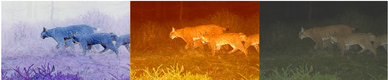
Figure 23: Example of color augmentations applied on the image (Left to right: image inversion, RGB shift, random brightness and contrast).
