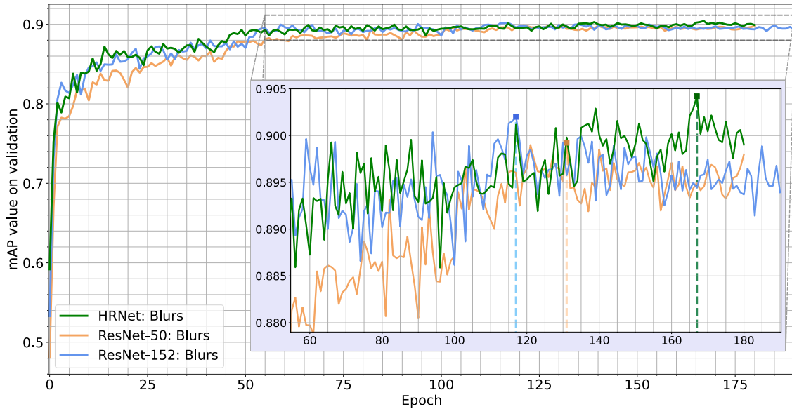
Figure 29: The comparison of validation mAP progression of the runs trained with the blur augmentations in the training image preparation pipeline.
