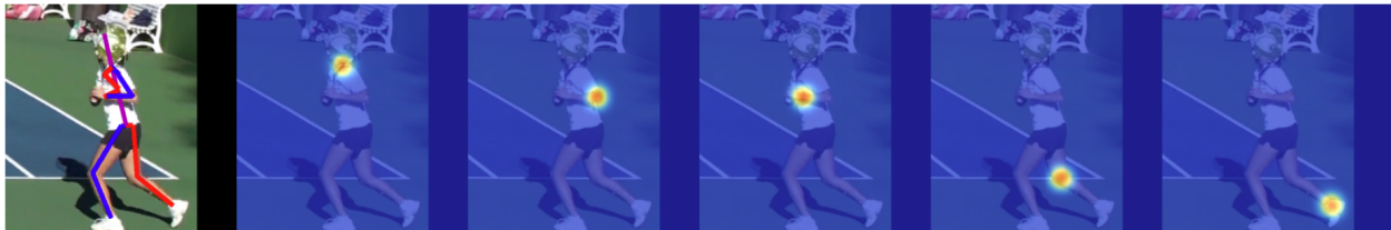
Figure 10: An example of heatmaps output from a CNN. The final pose estimation on the left is obtained as the maximum activation value of the heatmap [52].
