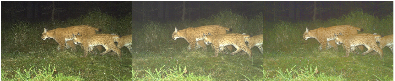
Figure 24: Example of noise augmentations applied on the image (Left to right: downscale, additive Gaussian noise, ISO noise).
