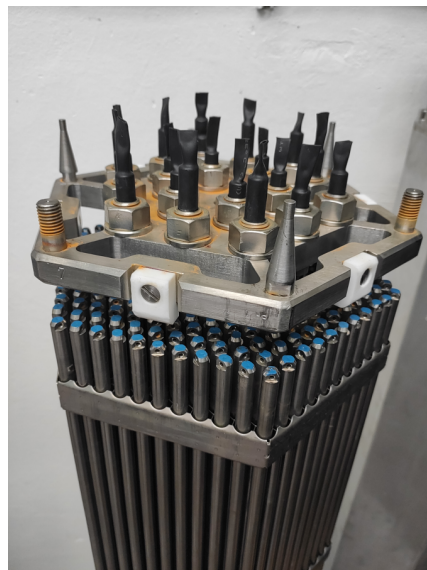
Fig. 4.11: Fuel assembly filled with absorber tubes, Case 4.
