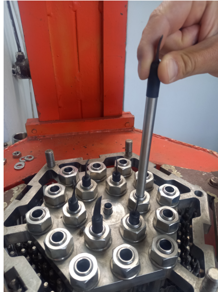
Fig. 4.10: Insertion of absorber tubes into the inner row of the fuel assembly.
