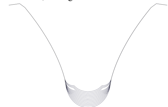
Fig. 8 Profiles of variants of the graded defect.
