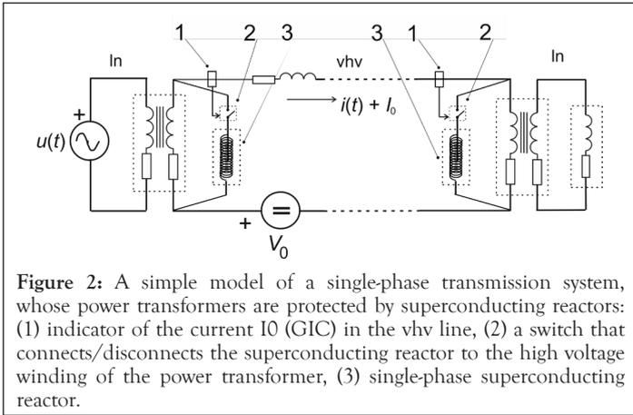
**Figure 2:** A simple model of a single-phase transmission system, whose power transformers are protected by superconducting reactors: (1) indicator of the current  $I_0$  (GIC) in the vhw line, (2) a switch that connects/disconnects the superconducting reactor to the high voltage winding of the power transformer, (3) single-phase superconducting reactor.
