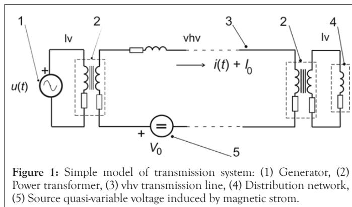
**Figure 1:** Simple model of transmission system: (1) Generator, (2) Power transformer, (3) vhv transmission line, (4) Distribution network, (5) Source quasi-variable voltage induced by magnetic storm.
