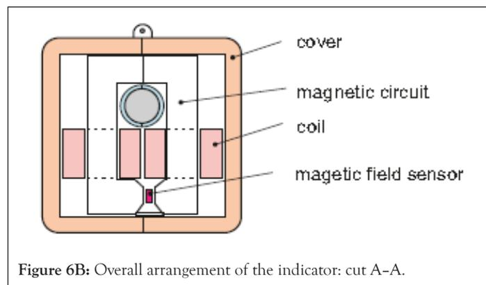
Figure 6B: Overall arrangement of the indicator: cut A-A.
