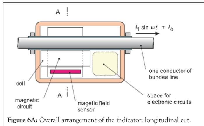
Figure 6A: Overall arrangement of the indicator: longitudinal cut.
