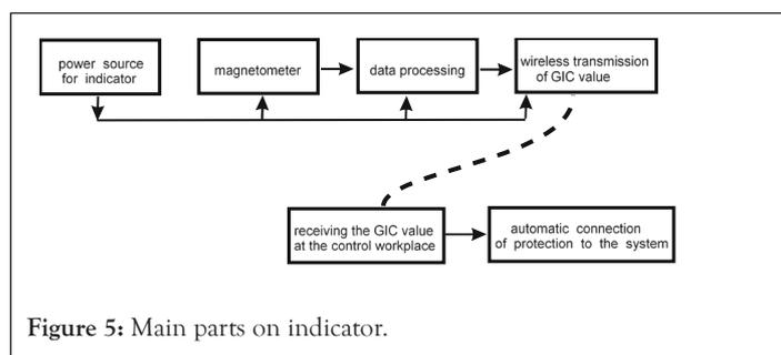
Figure 5: Main parts on indicator.
