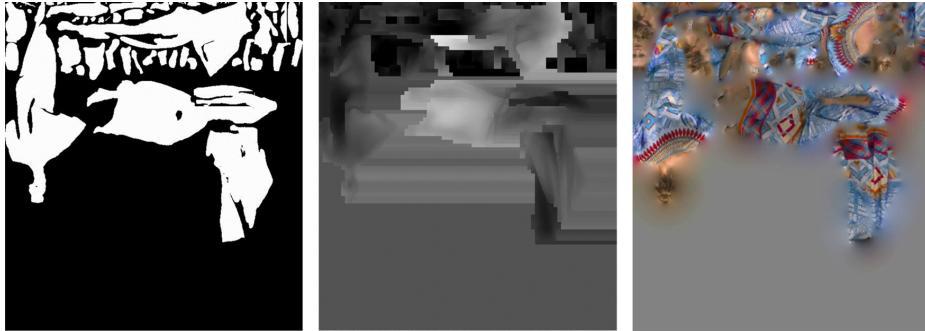
Figure 5.8: Example of the images encoded in V-PCC (from left to right): occupancy map, geometry image, attribute image. Source: [36]
