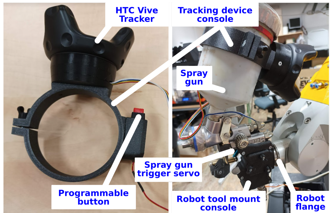
Figure 3. Tracking device console ( left ) with attached HTC Vive Tracker and programmable button, robot tool mount console ( right ) allowing installation of the tool to the robot flange for the automatic operation, here with the SATA jet 100 spray gun attached to a Fanuc arm.
