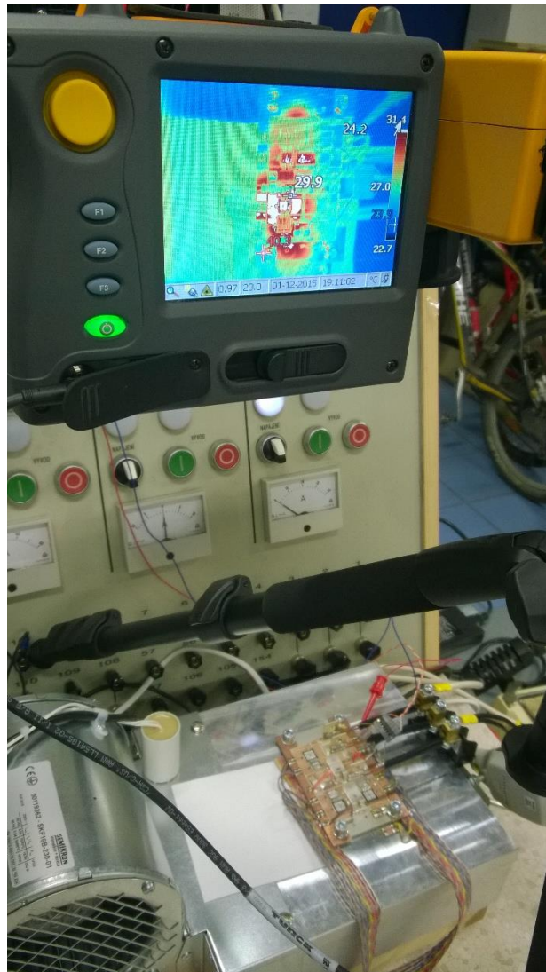
Figure 15: Infrared camera for measuring transistor and diode temperatures
