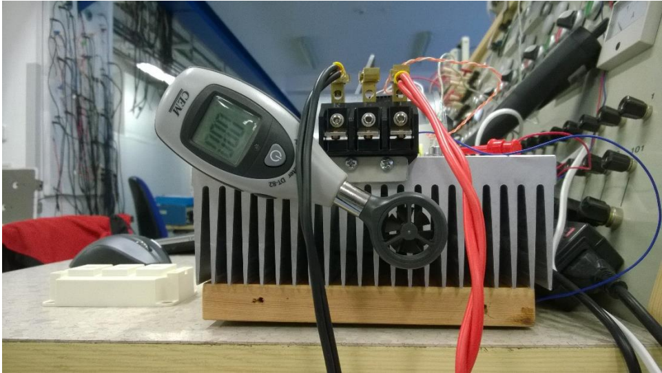
Figure 14: Anemometer used in measuring airflow rate
