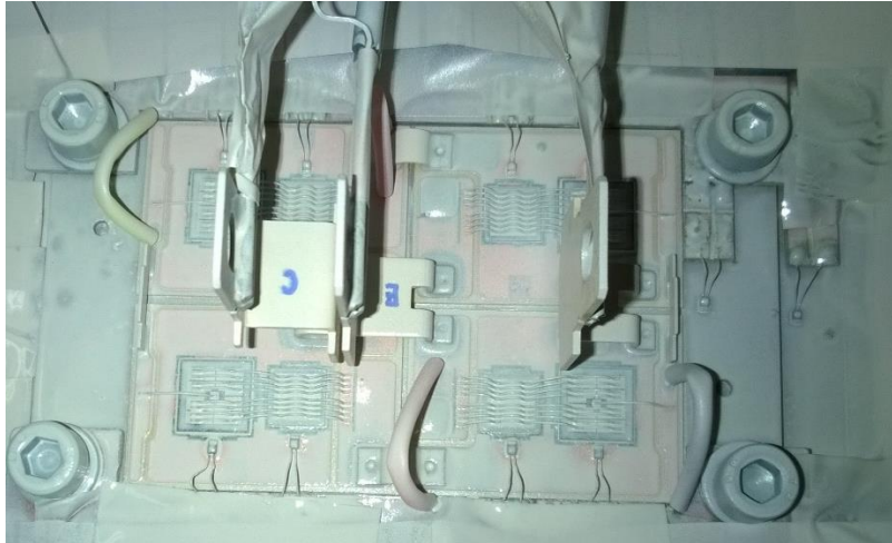
Figure 16: Opened IGBT module sprayed with thermal spray
