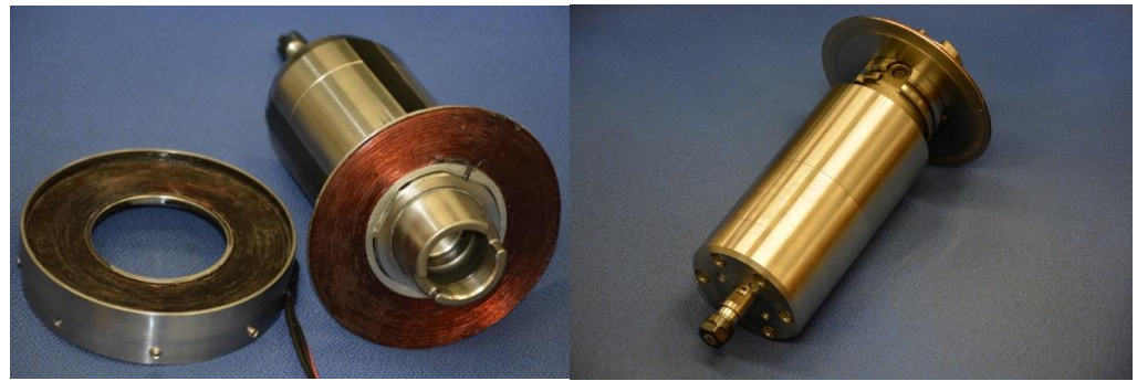
Figure 5. Magnetic couplers located at the top of the machining spindle clamping head.
