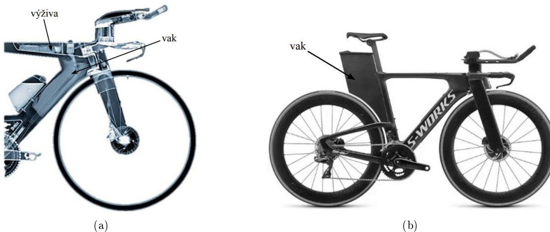
Obr. 6: (a) Detail uložení vaku modelu Canyon Speedmax [36], (b) Model Specialized Sworks Shiv [37]
