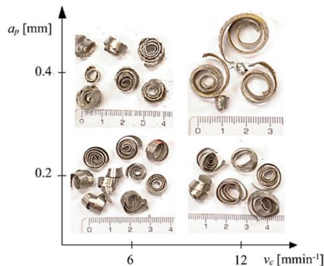
Figure 6. The shapes of chips and their dependence on cutting speed v_c and cutting depth a_p at tool angles for \gamma_o = 16^\circ , \lambda_s = 0^\circ , \kappa_r = 0^\circ .
