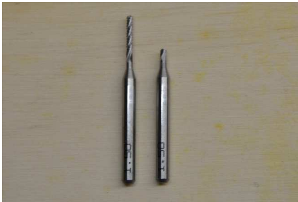
Fig. 1. Comparison of new and broken tool, 1.5 mm diameter
