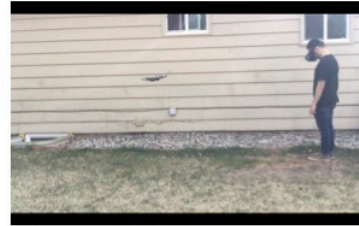
Figure 12: Tilting the head to the front, the drone moves to the front
