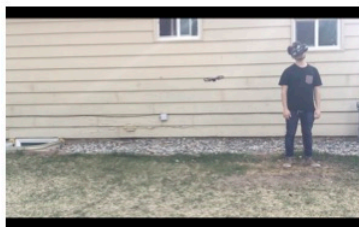
Figure 10: Tilting the head to the right, the drone moves to the right
