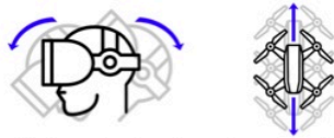
Figure 7: Tilting the head to the front/back, the drone moves to the front/back
