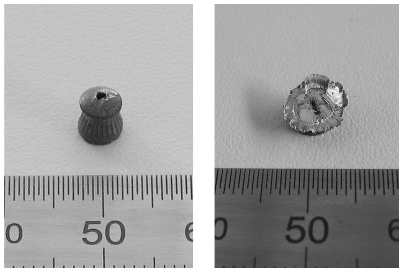
Fig. 8. Lead projectile (left – before impact, right – after impact)
