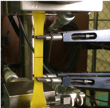
Fig. 5. Attachment of the external strain gauge
