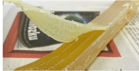
Fig. 4. Removal of the support material from three tension specimens
