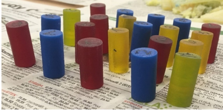
Fig. 3. Compression specimens printed vertically (ZXY); all colours
