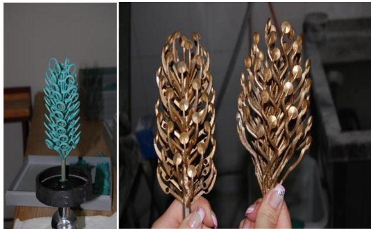
Fig. 1. Set of key castings for musical instruments. On the left, an example of a set of wax models, on the right an example of castings after removing the moulding compound [3]
