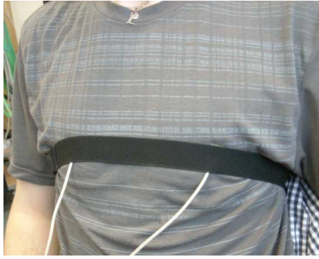
Figure 3. The capacitance electrodes placed on the T-shirt (under rubber belt)
