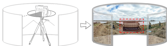
Figure 1: A demonstration of incorrect representations of dynamic objects (e.g. a running person) captured with an omnidirectional RGB-D scanning device.
