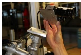
Figure 5: Camera dismantling with pinned fitting.
