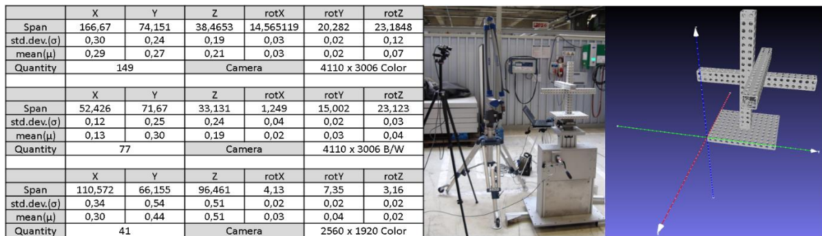
Figure 1: Results for Faro arm and test specimen. 3 different camera resolutions are used. Translations are in millimeters and rotations in degrees. Right: Experimental setup and scanned model of test object.
