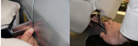
Figure 8 Laser line tool calibration to gaps.
