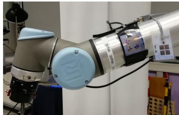
Fig. 5. Example of integration of the printed sensor on UR10 robot arm.
