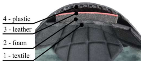
Fig. 2. Cross-section of shoulder protector
