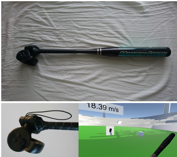
Figure 16: An Oculus Touch controller attached to the base of an aluminum baseball bat. We use this aggregate in a test conducted in a crude stadium scene with a pitching machine.
