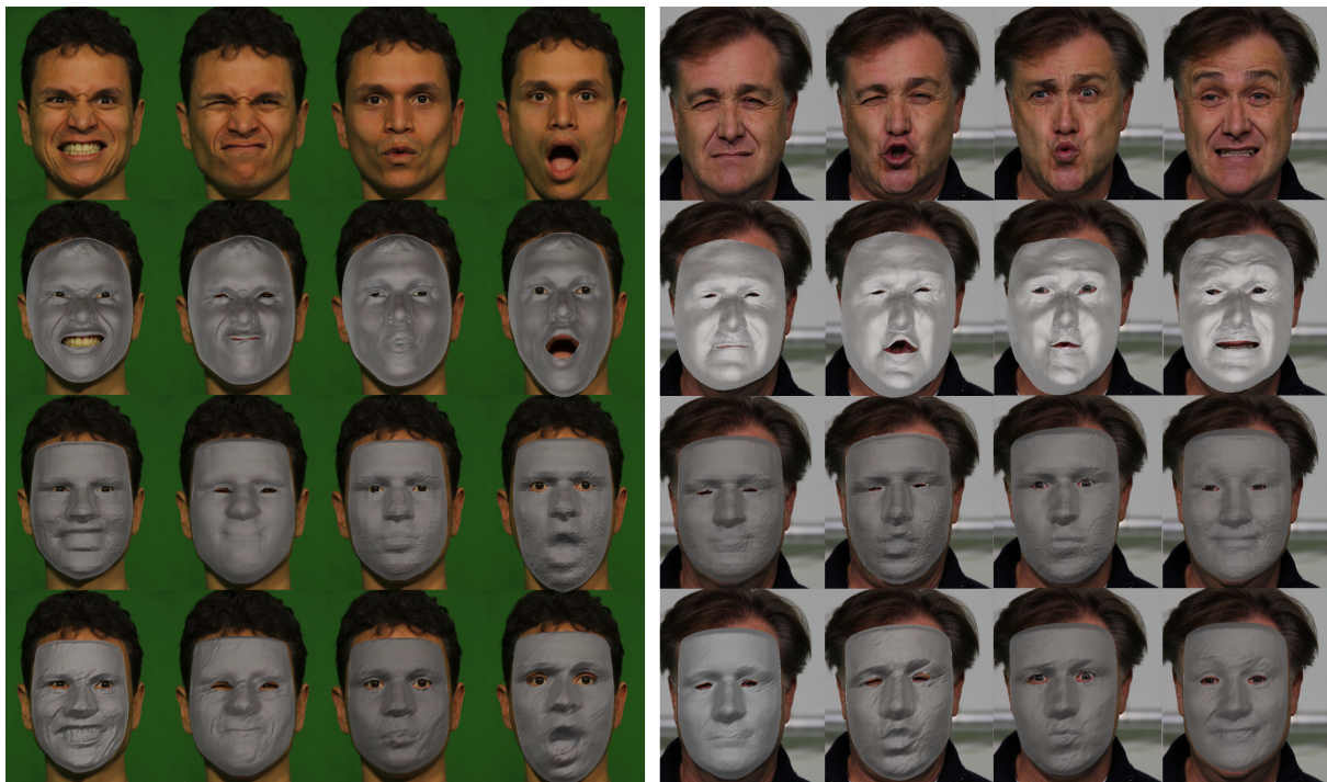
Figure 6: Detailed 3D reconstruction on real images. Left and right display the same. First row: Four input images at different expressions. From second to fourth row: Reprojected mesh of the 3D reconstruction using [GVWT13], [JBAT17] and ours, respectively. Note that the solution provided by [GVWT13] includes a 200k-point, instead of using 20k points like us.
