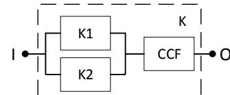
Figure 9. RBD of the robot contactors pair
