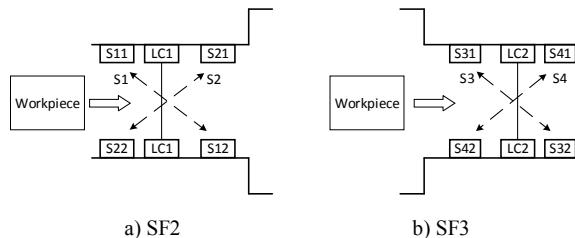
Figure 4. Principle of the sensor connection for the SF2 and SF3
