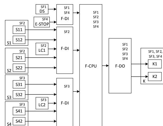
Figure 6. Assignment of safety functions to individual part of the SRS
