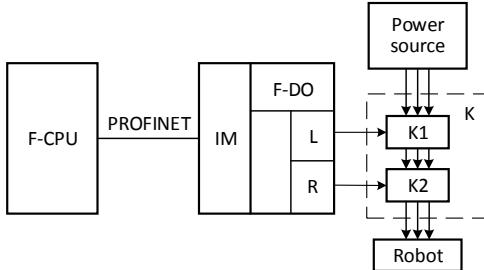
Figure 3. Principle of connection of the final elements block
