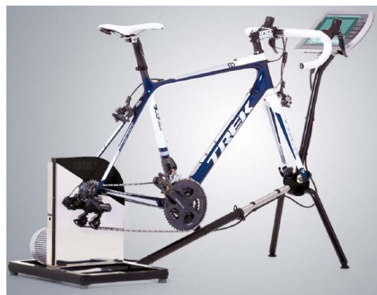
Figure 1. Example of ergometric bicycle for WAT test with control panel placed ahead from handlebars
