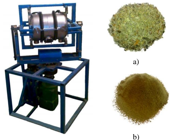
Fig. 1. Construction of a vibration equipment. Phytomixture material before a) and after b) processing.
