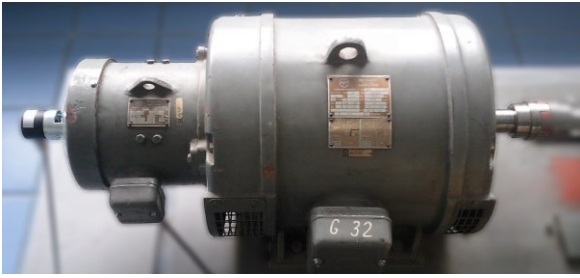
Figure 8. Laboratory WRSM with salient poles – 10kW
