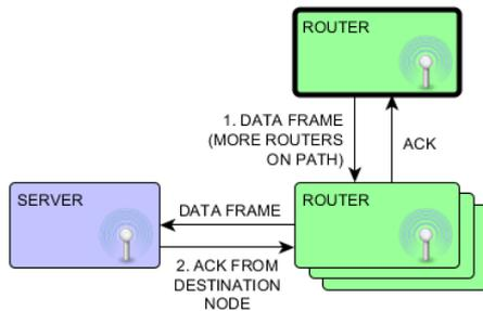
Figure 6 Delivering router to server communication
