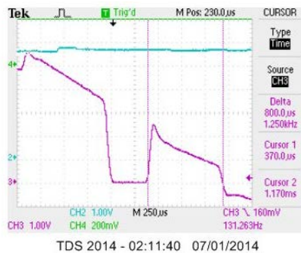
Figure 5-18: Commutation notch in the inverter (CMS) voltage
