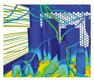
Fig.3: Pressure distribution and streamlines.
