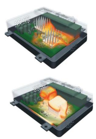
Fig.2: Base design (down) and optimized design (up) showing improved thermal behavior of a heat sink design.
