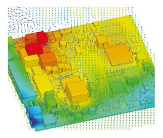
Fig.4: Temperature map and velocity vectors of PCB
