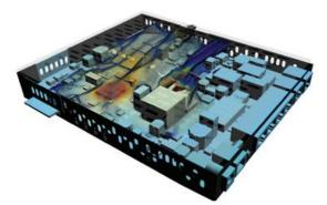
Fig.1: Chip temperatures and convention flow through a wireless router.
